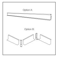
**3.**-Place the led light strip inside the led profile.(Depending on the desired size of the profile)
