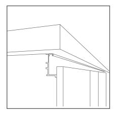
**8. Option B,** it is necessary to make a 45° cut in each corner and then place the connectors decorative exterior / interior
