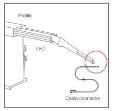
**11-** Next, connect the adapter depending on the inputs and then the power source to the light current
