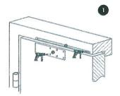
Use the supplied templates **0** to mark out the fixing holes for the door-closing mechanism and the sliding arm.
