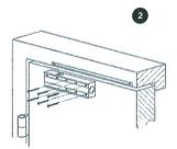
Screw the door-closing mechanism into position (in the standard assembly, the closing speed and end stop adjustment valves should be positioned between the door-closing mechanism shaft and the door hinge.
