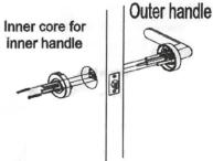
9.- Already having placed on the door latch, fasten with the screws the outside handle along with the inner core of the inside handle
