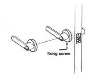
10.- Join the inside handle on the internal rosette and fixing screw
