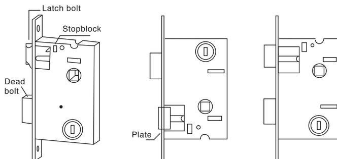
When installing the lock body, the latch bolt is on the upper side,
