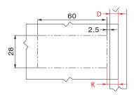
Use these formulas to determine the type of hinge arm, the drilling distance "K" and the height of the mounting plate "H" which is necessary to solve each application problem.
